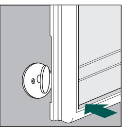
If you have a lever door handle and the handle extends over your door glass / door glass frame, the Enclosed Treatment unit may not fit. This interference issue is common with lever arm handles and window treatments. In order to make the Enclosed Treatment unit fit you will either have to change your door knob so that it does not extend over the door glass frame, or purchase a lever door handle extender.
