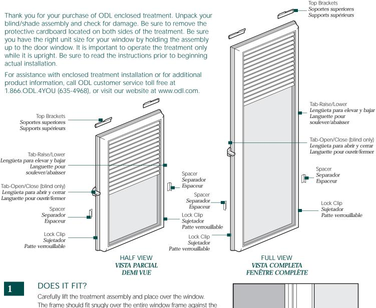
The frame should fit snugly over the entire window frame against the door. Look for anything that will prevent a flush fit or keep the treatment from functioning. Set the assembly down, standing it upright.
