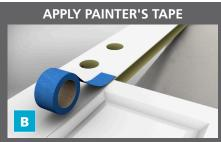
**B. APPLY PAINTER'S TAPE** around cutting area to prevent damage while cutting.
