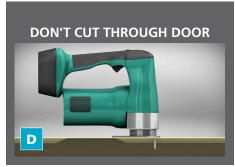
D. Do not attempt to cut all the way through the door. The up-stroke should not leave the door and the down-stroke should not exceed 1" into the door.
