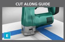
E. Using starter hole, **INSERT JIG SAW** with a shortstroke blade into the inner core of the door and **CUT ALONG MARKED GUIDELINES**, corner to corner.
