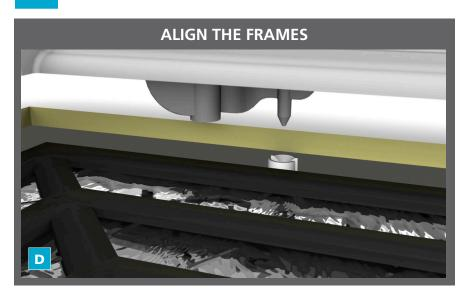
**D.** Align the frames by matching the screw hole guides.
