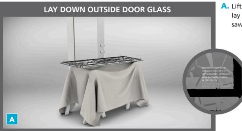
**A.** Lift the door off of the sawhorses and lay down the outside frame over the sawhorses, then add the glass overtop.
